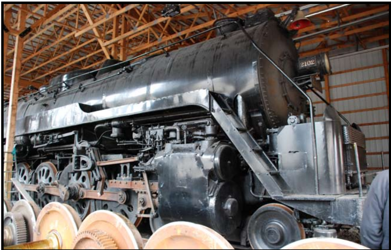
The former Reading Company 2102 steam engine. A Northern type locomotive with a 4-8-4 wheel arrangement.
